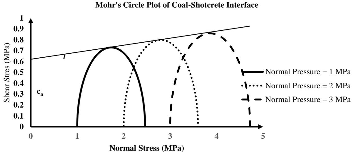
Figure 9: Mohr's Circle Plot of Coal-Shotcrete Interface
