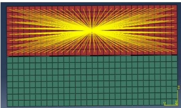
Figure 4: Numerical Model of Coal-Shotcrete Interface
