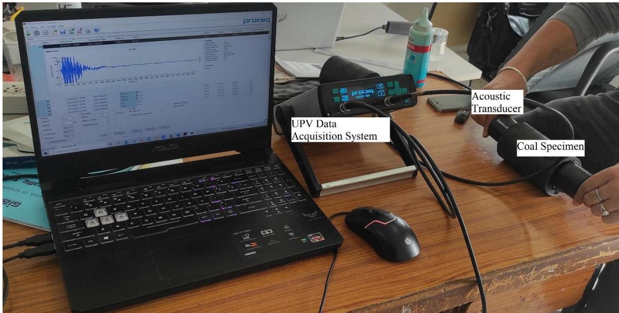
Figure 6: Ultrasonic Pulse Velocity Test
