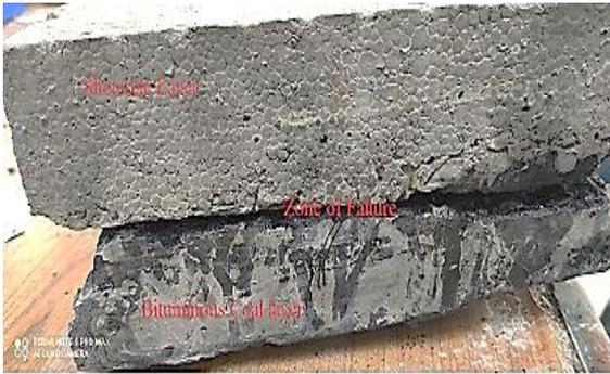
Figure 3: Coal-Shotcrete Interface Failure
