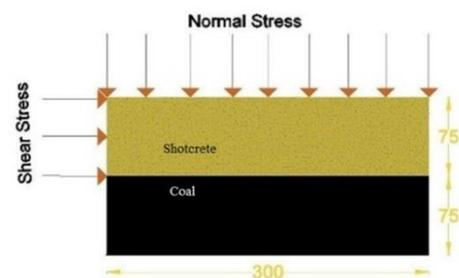
Figure 1: Stress State in Direct Shear Test
