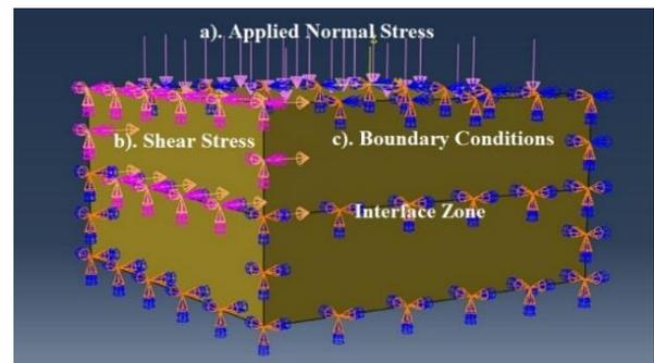
Figure 5: Depiction of a) Applied Normal Stress, b) Shear Stress and c) Boundary Conditions in Numerical Model
