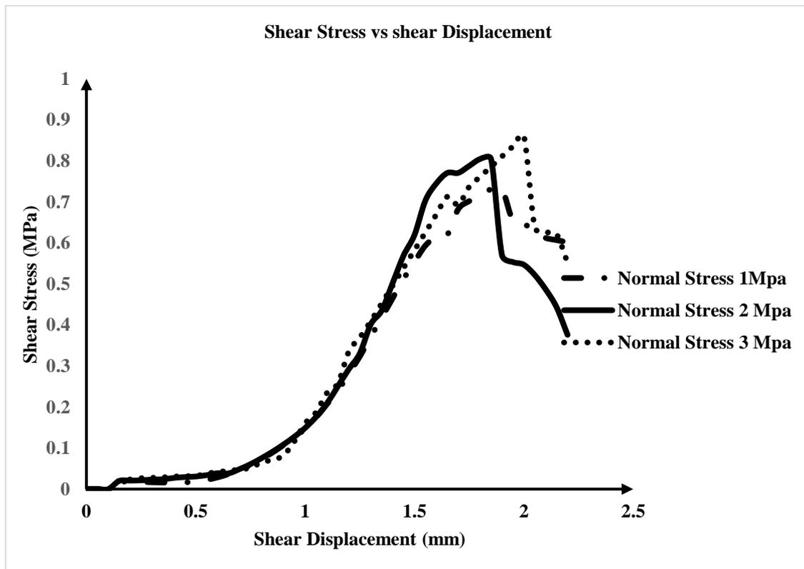
**Figure 8: Shear Stress Vs Shear Displacement of Coal-Shotcrete Specimens**
