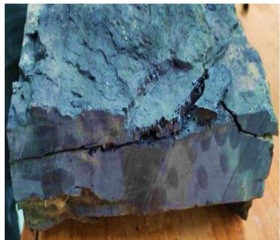
Figure 2: Failure State of Intact Coal Specimen
