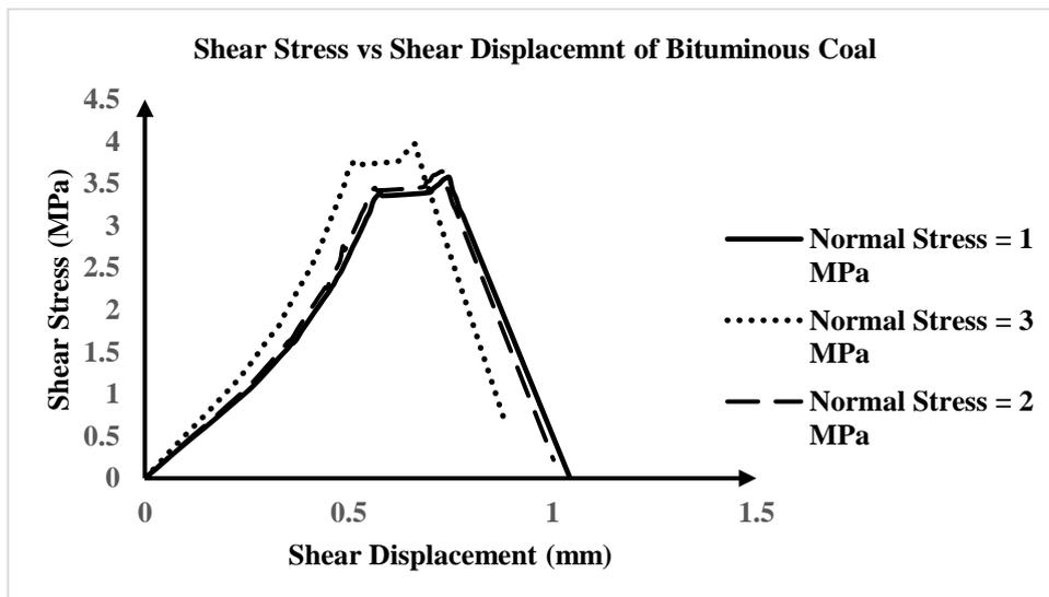
Figure 7: Shear Stress Vs Shear Displacement of Intact Coal Specimens
