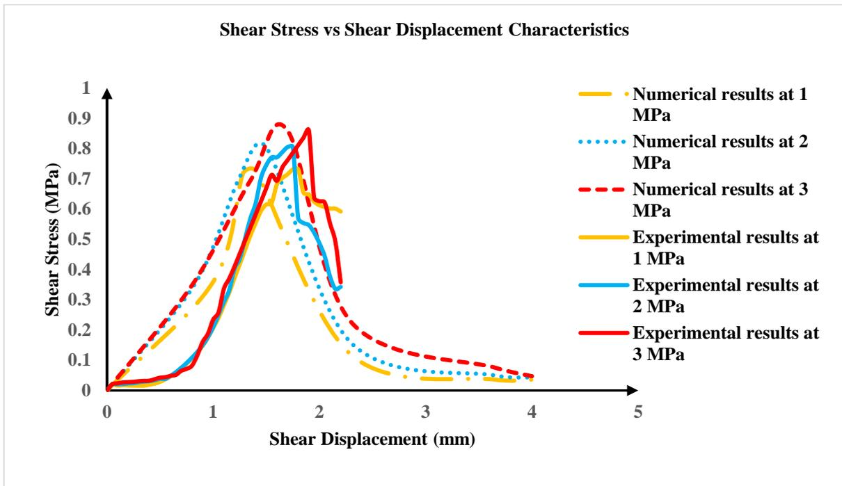
Figure 10: Experimental and Numerical Results of Shear Stress Vs Shear Displacement of Coal-Shotcrete Interface
